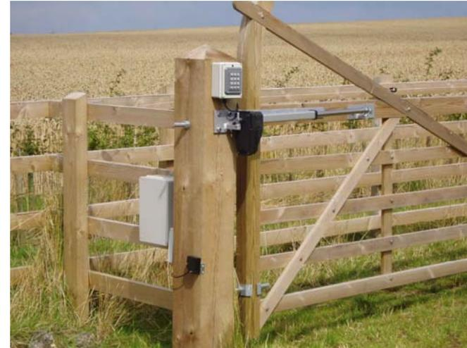
Hollin Applications, have designed this control to remotely operate a gate using a Danaher Thomson Industrial Linear Actuator.
