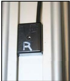
The stroke can be adjusted on the LA14 actuator by sliding the magnetic limit switches on the side of the Actuator. These are locked in place with a tiny grub screw, use the 1.5mm allen key provided.
