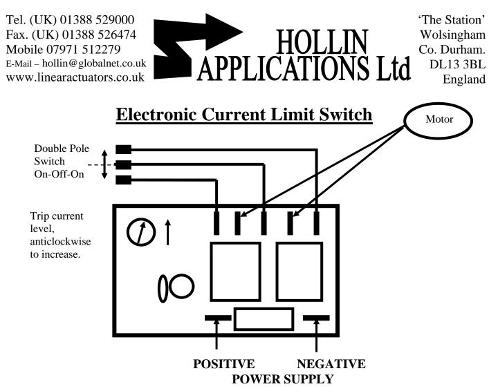
This circuit designed by Hollin Applications uses an input signal to switch the direction of a linear Actuator. The double pole switch changes relays in a H-Bridge configuration which changes the direction of current flow and shorts the D.C. Motor when switched off. This ensures a minimal amount of overrun on the Actuator. This circuit automatically converts the low power input signal to the high current motor drive.
